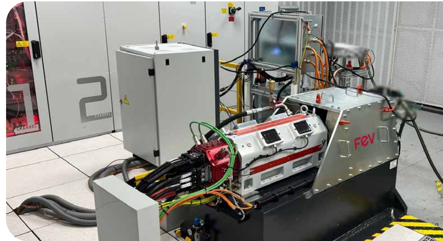
Dynamic E-Motor test bench of 24 000 rpm and above: good accuracy for speed control for low speed (0..10 rpm)
